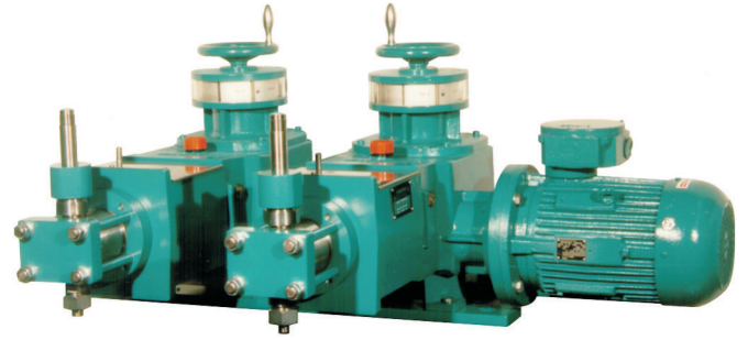
2-headed PIM M plunger-metering-pump with stroke adjustment by hand-wheels and with stuffing boxes and lantern rings
